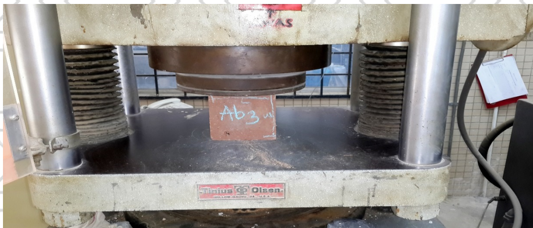
Figure 2.14: Stabilised earth block Specimen in a Compressing Machine
