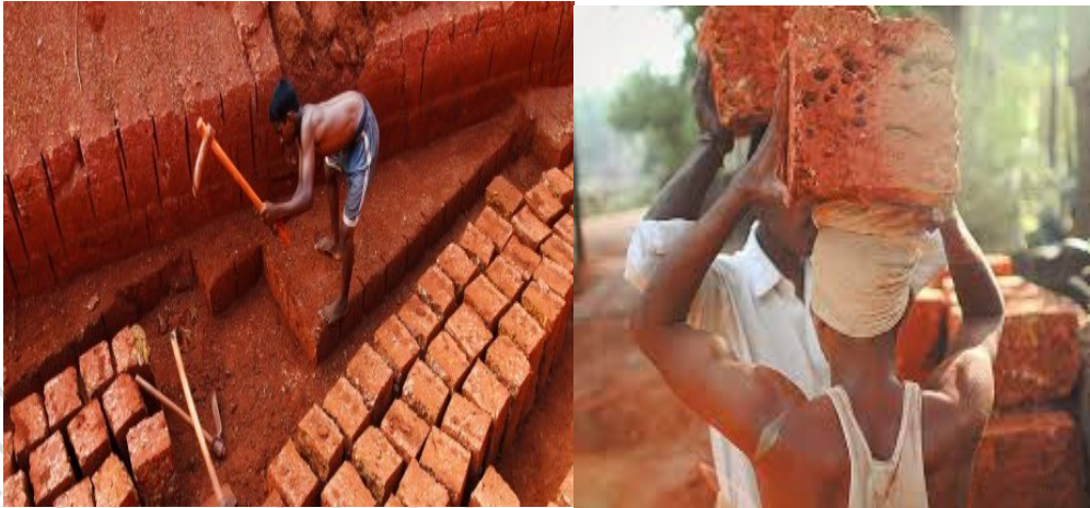
Figure 2.3: Locally Sourced Laterite Soil Cut Out in Block Shape and Taken for Firing.
